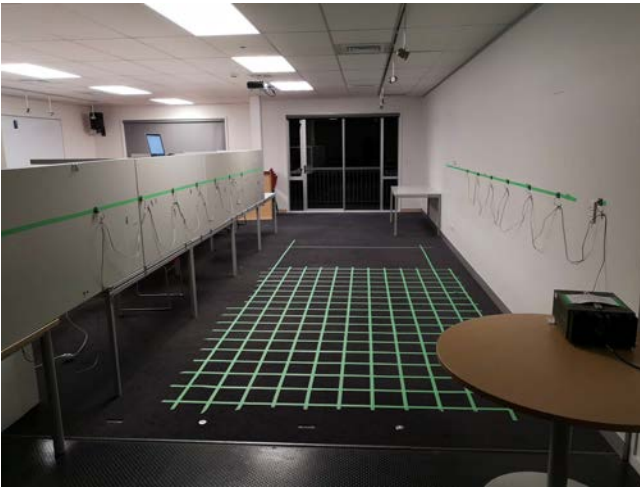
Fig. 5. Experimental setup showing the wall mounted light-sensors and the test space.
