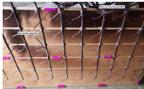
Fig. 2: Copper floor sensing tiles. Each tile is connected to a microcontroller with a wire.
